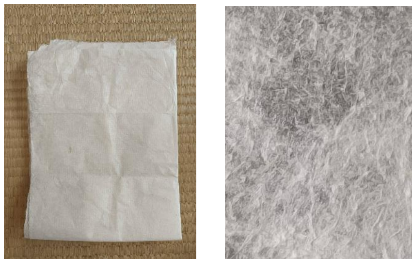
Figure 4 Appearance of (left) pineapple paper and (right) pineapple fiber when viewed with a 10x magnification
